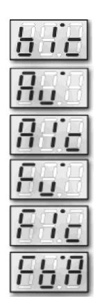
**Bulk Time.** Controls the minimum time period for non-calculated bulk charging. Standard value set by battery program selected. Adjustment spans in tenths of hours from 12 minutes to six hours. To reverse direction of scroll, release magnet and wait for LED to display b1c code. Re-activate switch with magnet and release when desired value is indicated.
