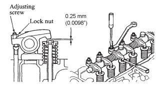
Figure 9: Valve Adjustment
