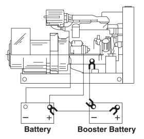
Figure 12: Booster Battery Connections
