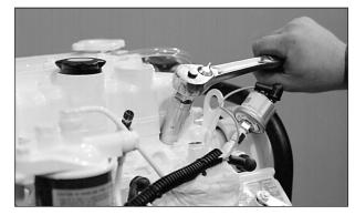
Figure 18: Unscrew injector.
