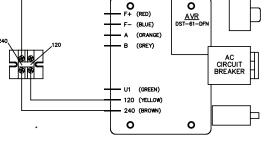
Figure 30: Control Terminal Board, 120/240 Volt Output
