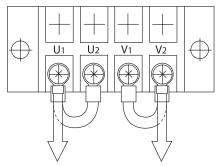
Figure 27: Output Terminal Board, 120 Volt Output
