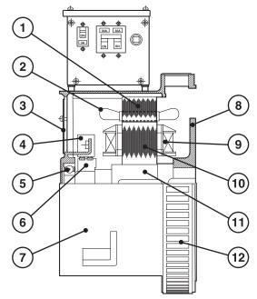
Figure 24: Generator Components.
