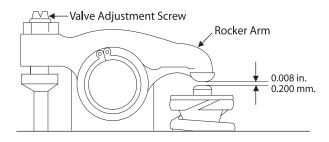
Figure 10: Valve Adjustment
