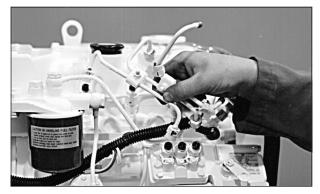
Figure 14: Remove delivery lines.
