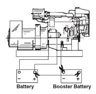
*Figure 22: Battery connections.*
