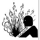
not remove a filler cap unless it is cool enough to comfortably grip with bare hands. Slowly loosen cap to relieve pressure before opening fully.
