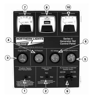
Figure 6: Series 4 Generator Control Panel
