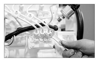
Figure 13: Remove delivery line flare nuts.
