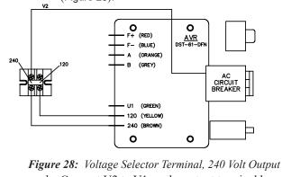
3. 120/240 Volt Output a. Connect the control terminal board for 240 volts (Figure 30).  $V^2$   $F^+$  (RED)  $F^-$  (BLUE) A (ORANGE) B (OREY)  $F^-$  (BLUE)  $F^-$  (BLUE) F
