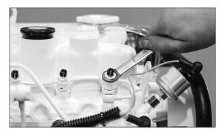
Figure 16: Remove return line nuts.
