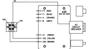
Figure 26: Control Terminal Board, 120 Volt Output
