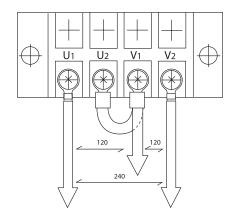
b. Connect U2 to V1 on the output terminal board (Figure 29).
