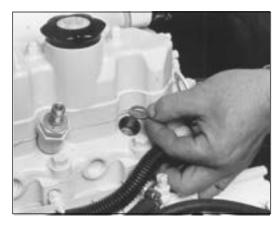
Figure 15: Remove and replace copper sealing washer.
