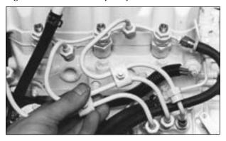
Figure 11: Remove delivery lines.
