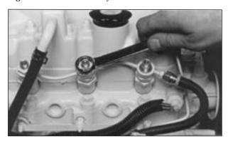
Figure 12: Remove return line nuts.
