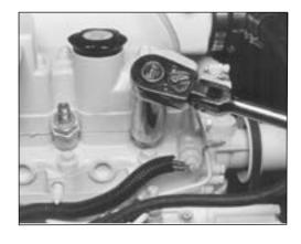
Figure 14: Unscrew injector.
