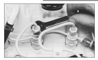
Figure 10: Remove delivery line flare nuts.
