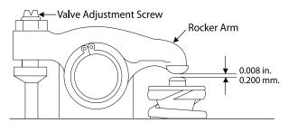
Figure 8: Valve Adjustment
