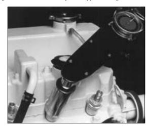
Figure 16: Reinstall injector. Torque to proper tightness.
