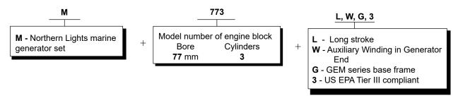
M773LW3 = Northern Lights marine generator set with a 773 engine, PX-309K2 generator end, AVR, US EPA Tier III.
