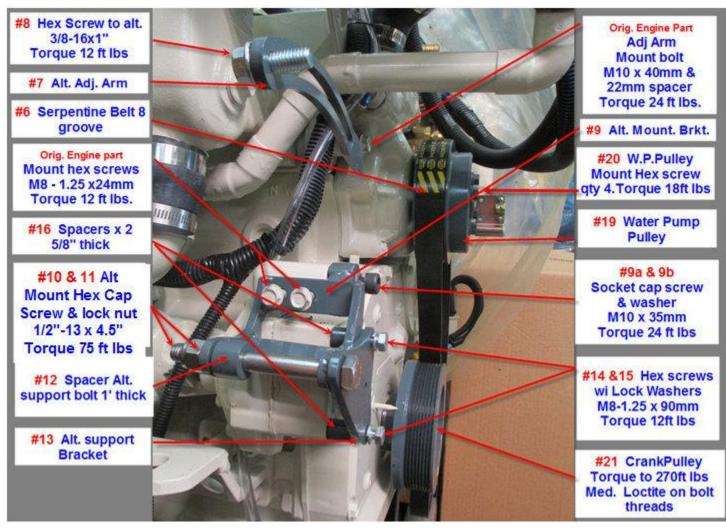
REFERENCE NUMBERS, FASTENER SIZES, AND TORQUE SETTINGS
