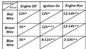
\* 11.5 - 12.8 VDC battery voltage at rest (no charging occurring). If your batteries are isolated and your RED (sensing) wire shows voltages other than those shown above, make sure that the wire is connected on the "battery" side of the isolator. The red wire must "see" the battery directly. \*\* 13.5 - 14.5 VDC battery voltage when charging.
