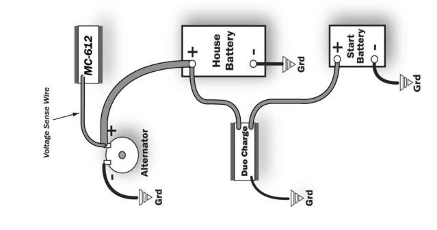
House / Start Battery Banks - With Centerfielder & Duo Charge Twin Engines / Dual Alternators / Dual Regulators
