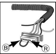
*Figure 24 - Jumping power wire to field.*
