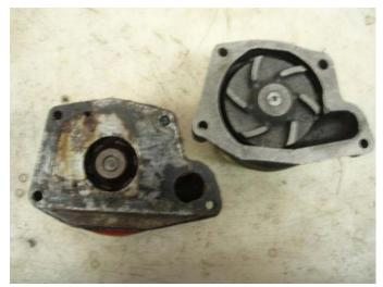
14. Old and new pumps are shown side-by-side. The gasket plate between the old pump and engine block will need to be removed, cleaned, and re-installed with the new pump.
