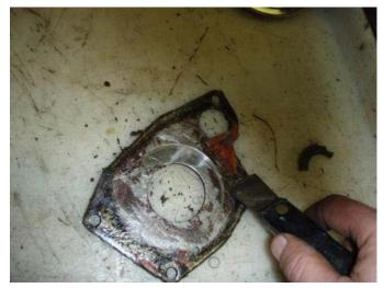
16. The gasket plate must be free of any old sealants of any other foreign matter before re-installation. Don't take any shortcuts during this process.
