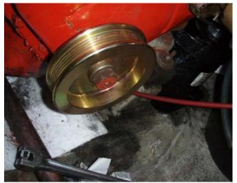
11. Completed serpentine crank shaft pulley.
