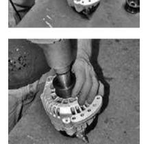
5. Re-attach wiring to alternator.
