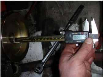
9. When seated, the serpentine crank pulley will extend approximately 1/4" forward of the crankshaft.
