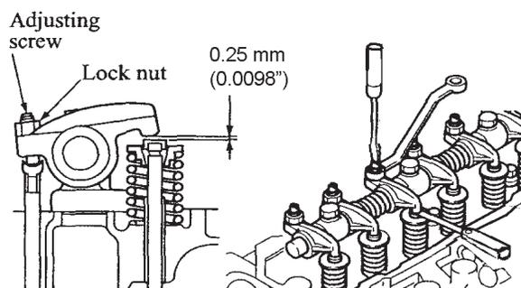
*Figure 9: Valve Adjustment*
