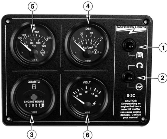
Figure 5: Series 3 Generator Control Panel
