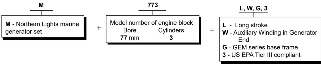
**M773LW3** = Northern Lights marine generator set with a 773 engine, PX-309K2 generator end, AVR, US EPA Tier III.
