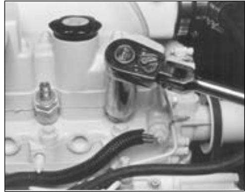
**Figure 14:** Unscrew injector.
