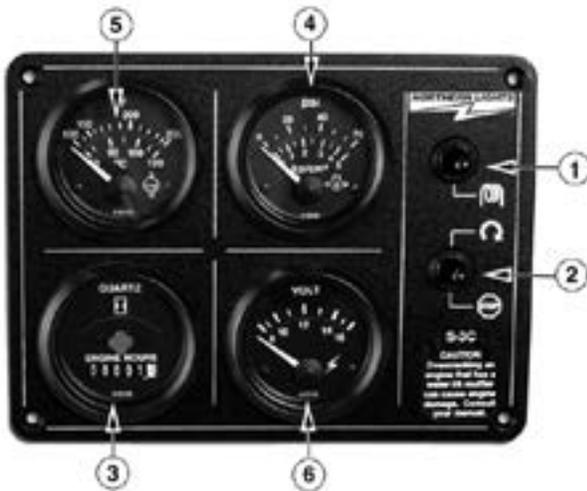
Figure 6: Series 3 Generator Control Panel
