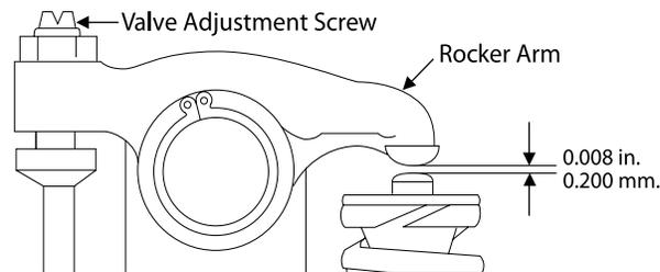
**Figure 8:** Valve Adjustment
