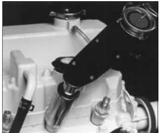
**Figure 16:** Reinstall injector. Torque to proper tightness.
