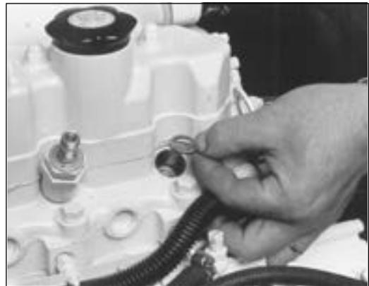
**Figure 15:** Remove and replace copper sealing washer.
