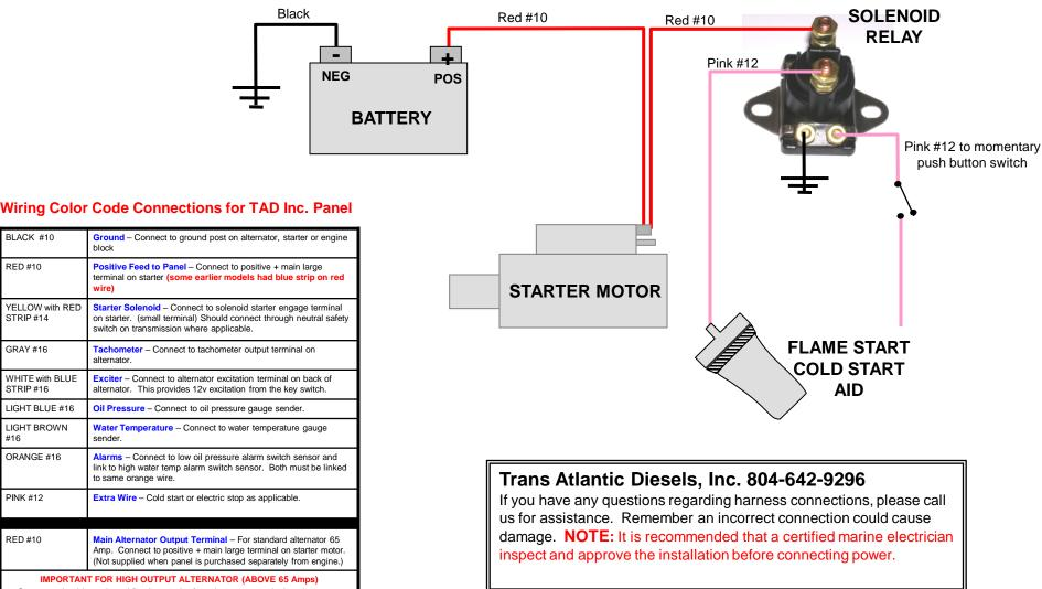
Customer should supply and fit a larger wire from the output terminal on the alternator to the battery/s directly or via main Positive terminal on starter motor. Wire sized according to output and length of wire. If the alternator is isolated ground, than the size of the ground wire should also be increased. Contact alternator manufacturer for recommendations on wire size. Standard #10 Red wire in harness is only suitable for standard 65 amp alternator.
