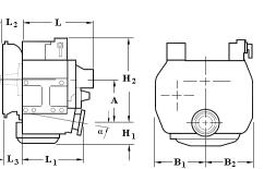
mm (inches) Bell B<sub>1</sub> B<sub>2</sub> H<sub>2</sub> Angle Α H<sub>1</sub> L L L<sub>2</sub> L<sub>3</sub> Hsg. 7.0 149 (5.87) 215 (8.46) 215 (8.46) 126 (4.96) 315 (12.4) 418 (16.5) 300 (11.8) 55.0 (2.16) 35.5 (1.40) Weight kg (lb) Oil Capacity Litre (US qt) 77.0 (170) 5.00 (5.32)
