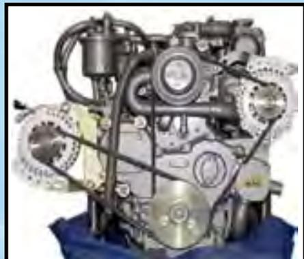
for balanced charge control over dual alternators. By monitoring port and starboard alternators and regulators, and controlling field output to both alternators, the Centerfielder II makes it possible to direct the combined output from both alternators to charge a central house battery bank.
