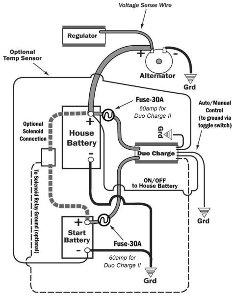
**Voltage Sensing**: Alternator and regulator supply house bank only. Sense at house battery's positive post or at the positive output of the alternator.
